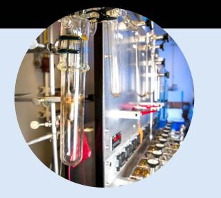
Our high-vacuum fluorination system converts uranium oxides into O<sub>2</sub> gas for isotope ratio analysis, and facilitates synthesis of actinide compounds of interest to our nonproliferation mission. We also use a laser-heated fluorination capability, which reduces sample size requirements and increases throughput.
