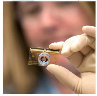
The "human on a chip" microphysiological systems integrates biology and engineering with a combination of microfluidics and multi-electrode arrays to model human responses.
