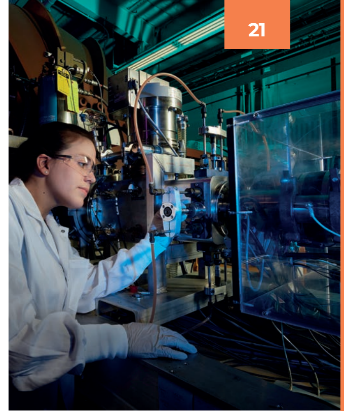
At LLNL's Center for Accelerator Mass Spectrometry, a suite of unique instrumentation enables scientists to analyze radioactive isotopes in bio-based samples, providing insight regarding the age of unknown biological material.
