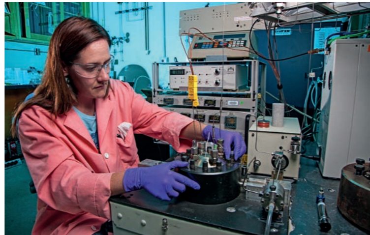
A researcher prepares a rock sample for a core-flooding experiment to test its response to carbon dioxide exposure under reservoir temperature and pressure conditions.
