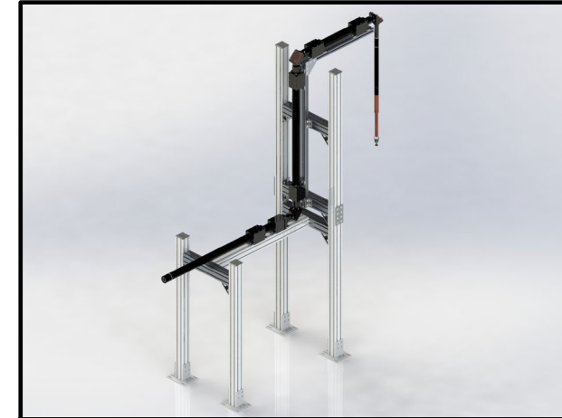
Overmoded corrugated waveguide line from gyrotron to an NMR probe
