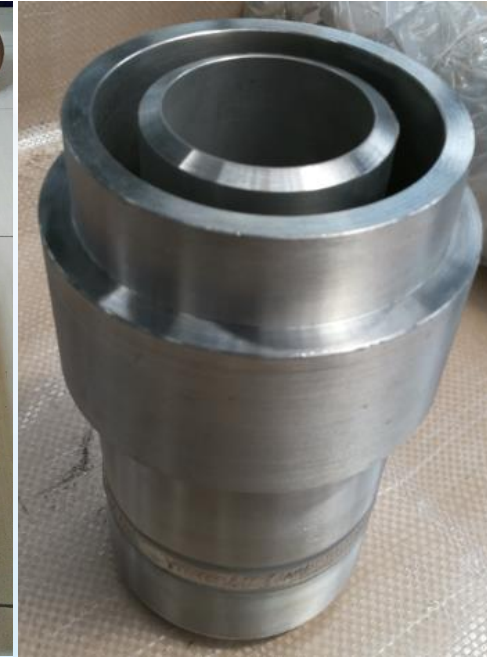
Prototype mockup of double-layer pipe for shield
