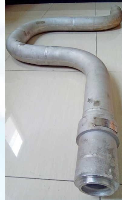
Prototype mockup of double-layer pipe for shield
