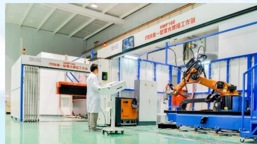
(5) 16kW laser welding into use, realizing full-penetration welding without back sputtering
