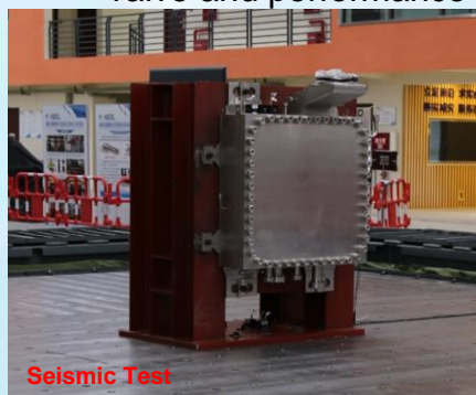
GF GVB shell trail-manufacture and design conformity tests.
