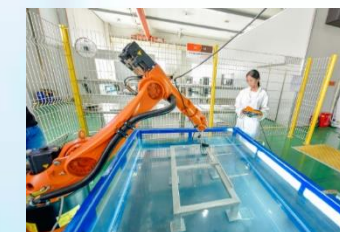
(6) Phase-array UT, developing creep-wave technique
