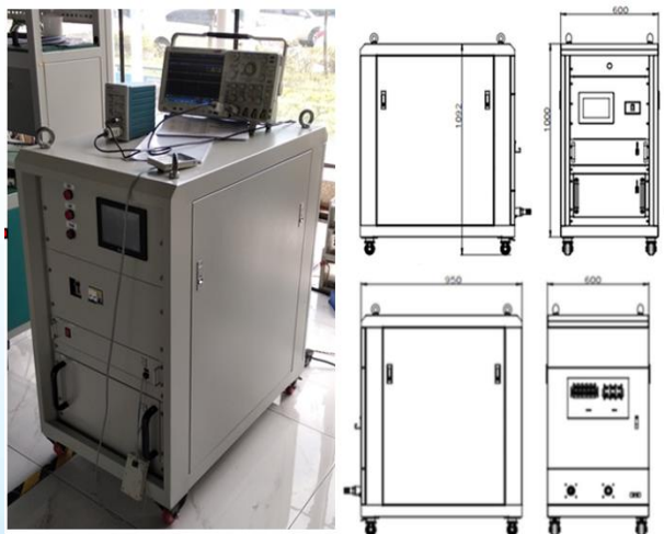
Mock-up of GDC Power Supply
