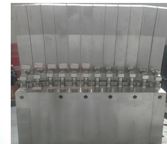
(8) Assembly 12 dummy fingers with a central beam
