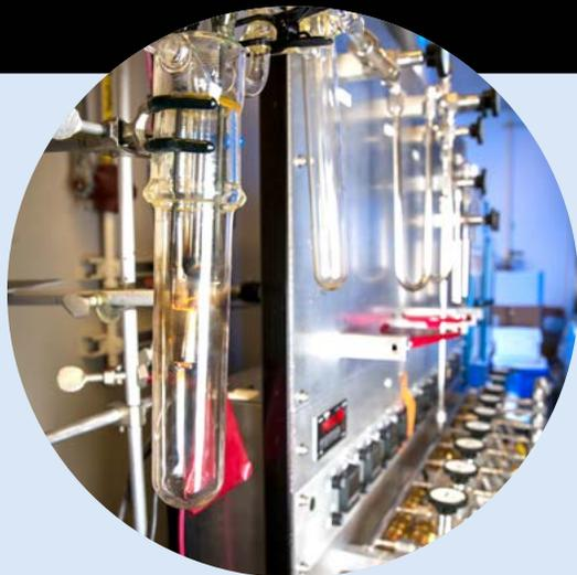
*Our high-vacuum fluorination system converts uranium oxides into O<sub>2</sub> gas for isotope ratio analysis, and facilitates synthesis of actinide compounds of interest to our nonproliferation mission. We also use a laser-heated fluorination capability, which reduces sample size requirements and increases throughput.*
